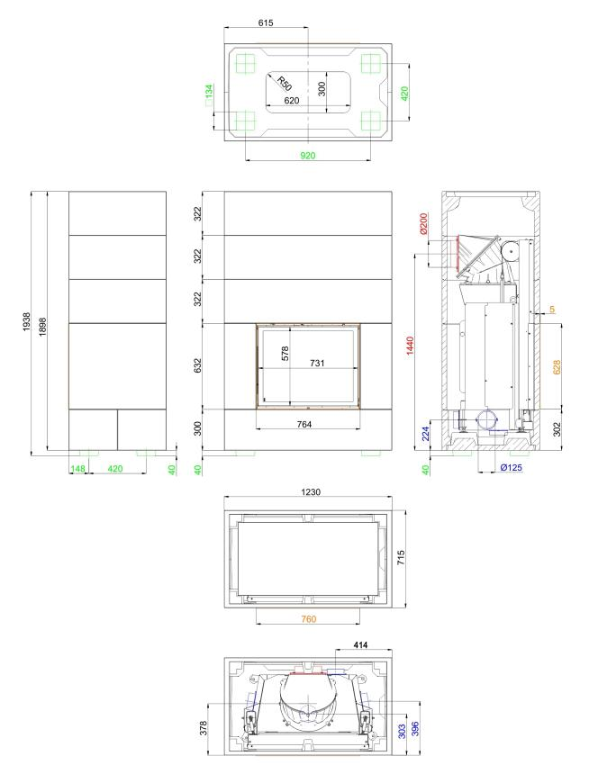
frame (orange), combustion air nozzle (blue), levelling feet (green) marked in color
